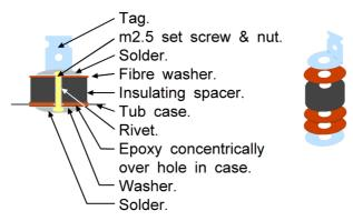
NB epoxy 2 fibre washers to spacer before assembling.
